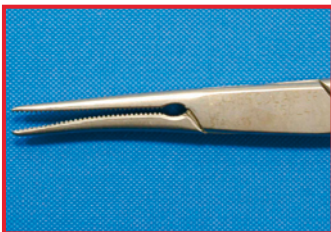
Deformation caused by improper handling
