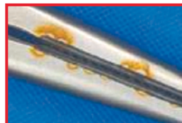
Etching effect on soldered seams. On hard-metal scissors, hard-metal tweezers and needle holders Cause: Effects of acid due to over-dosing of neutralizing chemicals or due to using acid-based cleaners.
