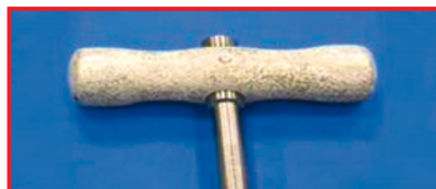
Material affected at aluminum handle Cause: Unsuitable alkaline cleaner
