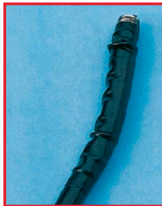
Swollen insertion tube caused by using unsuitable care agent.
