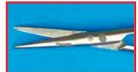
Partial etching effect and deposits of an etching agent causing hemostasis on the surface of the instrument. Causes: contact time too long
