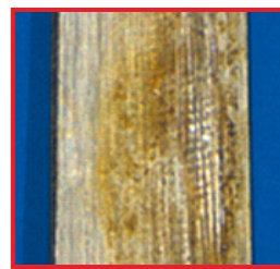
Bone punch, friction surface on sliding section indicates onset of friction corrosion..
