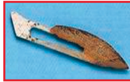
Surface of blade affected due to humidity. Causes: Composition of materials, normal steel, so disposable product.
