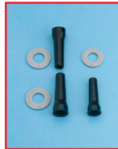
Right: Swollen seals caused by incorrectly applied instrument oil. Left: New seals
