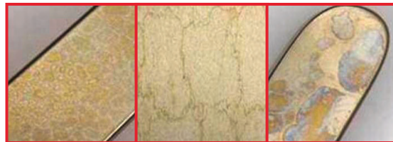
Typical silicate discoloration on the surface of the instrument after steam sterilization caused by excessive silicic acid levels in the demineralized water.
