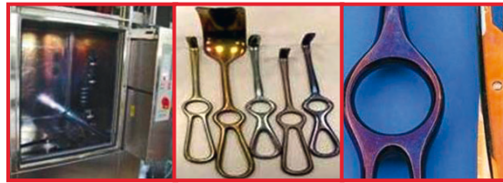
Typical silicate discoloration in the rinsing chamber and on the surface of the instrument caused by cleaning agent containing silicate, or excessive levels of silicic acid in the water.
