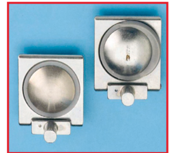
Right: Leaking flap valve on a trocar caused by the seal swelling as a consequence of contact with oil. Left: New flap valve
