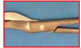
Etching effect on surface of instrument. Causes: Effects of over-dosed acids.
