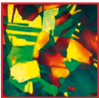
Color etching - austenitic microstructure on corrosion and acid-resistant instrument steel (magnified 500 times)
