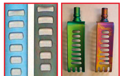
Section - titan valves: Left-hand Valve – brand new. Right-hand valve – machine-cleaned. The change in color is generally even. However it can also occur in patches.
