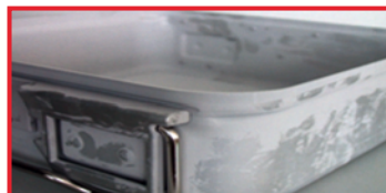
Material affected on natural/colored anodized aluminum surface of containers. Causes: alkaline washer solution above permitted level
