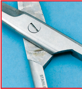
Fretting corrosion due to inadequate lubrication
