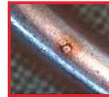
Pitting on tweezers. Causes: Over-aging of color-coding band allows harmful substances containing chloride to infiltrate.
