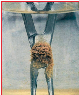
Corrosion caused by immersion in physiological salt solution over a period of several hours
