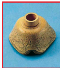
Aging tear in a breathing mask
