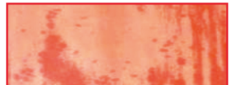
Material affected on natural/colored anodized aluminum surface of containers. Causes: alkaline washer solution above permitted level
