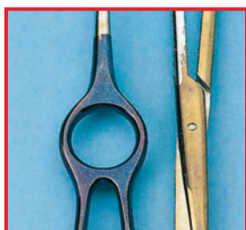
Instruments discolored by silicic acid
