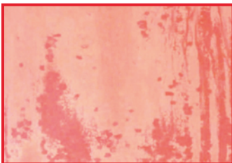
Optical changes to color anodized aluminum occurs even in mildly alkaline solutions
